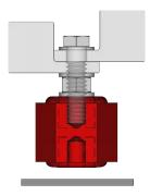
3) Bolt up the standoff bottom mounting bolt
